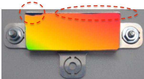
Separation of the coating on the FUV grating – Qualification model
